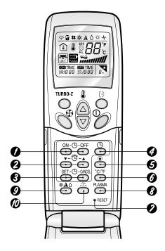
**ON/OFF TIMER BUTTONS** Used to set the time of starting and
